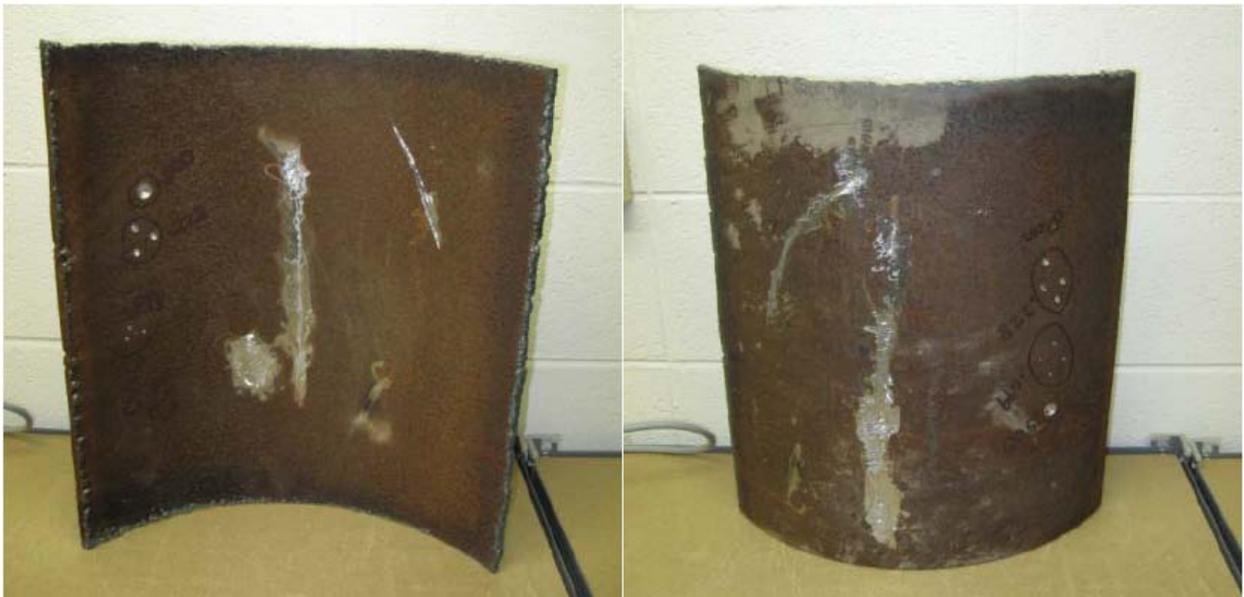
**Figure 22. 24 inch diameter steel pipe (left) sample 1, internal defects; (right) sample 2, external defects.**
