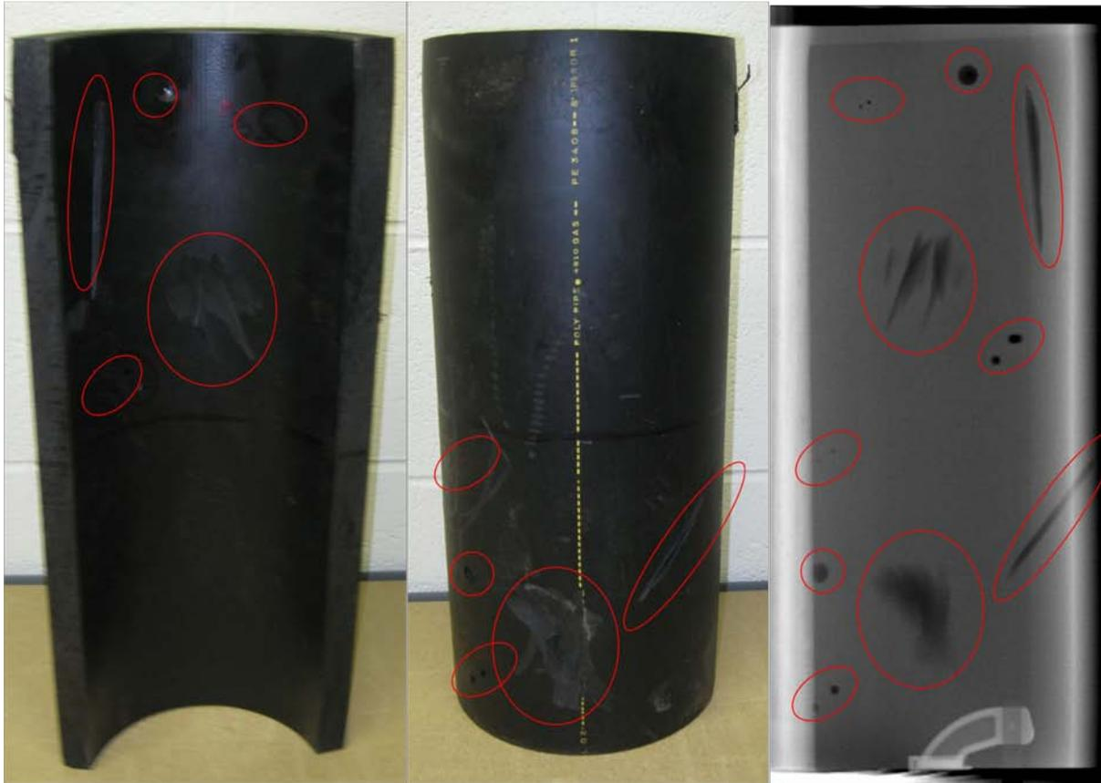
**Figure 31. Sample RSD scan of 8 inch diameter Polypipe, HDPE, 3408.**
