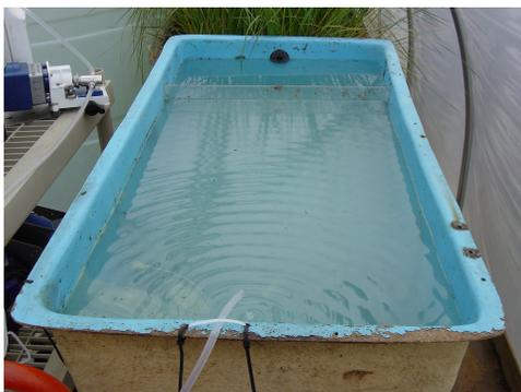
**Figure 26:** Oil/Water Separator used in Experiment 3.
