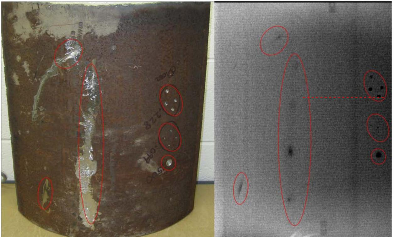
Figure 25. Sample scan of  $\frac{1}{4}$  inch wall steel pipe, external defects, 160 kV. Note the pipe was imaged from inside out so the defects are mirror imaged.
