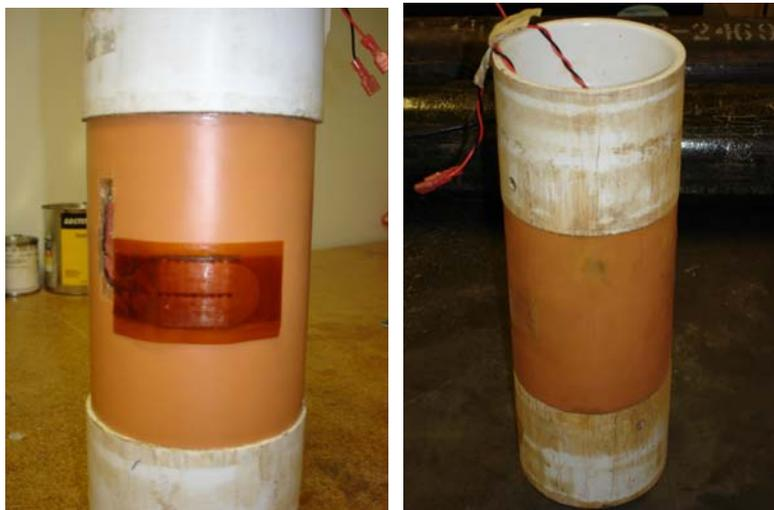
**Figure 22** Left: 1<sup>st</sup> generation tool with sensors installed. Right: after installation of the wear-resistant coating.
