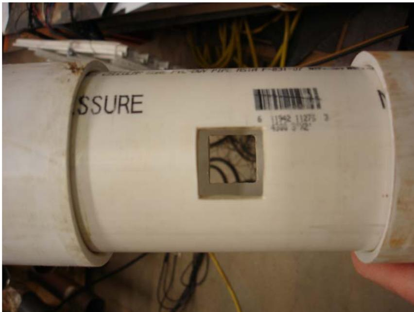
**Figure 20** 3.5 in. prototype tool skeleton with 4 in. couplers on each end and diametrically opposing holes to accommodate EMAT sensors.
