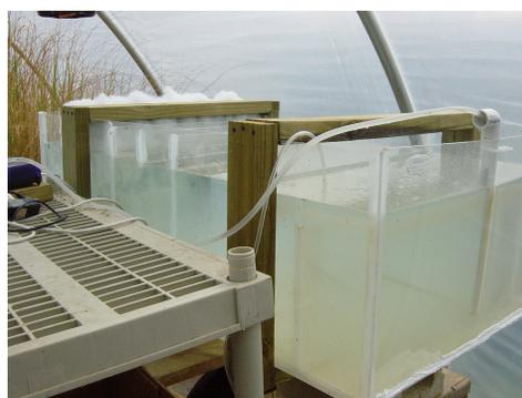
**Figure 27:** Newly constructed Oil/Water Separator used in Experiment 4.
