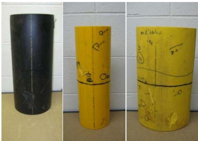
**Figure 21. Poly pipes include a combination of polyethylene and polyamide pipes: (left) 8 inch diameter Polypipe, HDPE, 3408; (center) 6 inch diameter, Polyamide 12, SDR 11; ( right) 12 inch diameter, DriscoPlex 6500 PE 2406, MDPE.**
