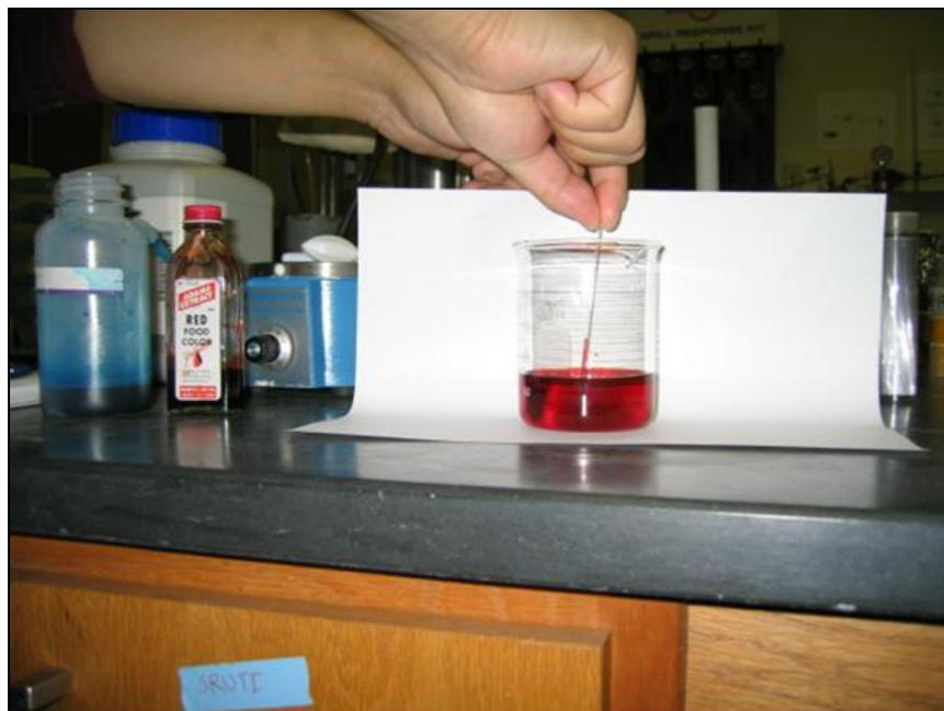
**Figure 1. Capillary tube test.**
