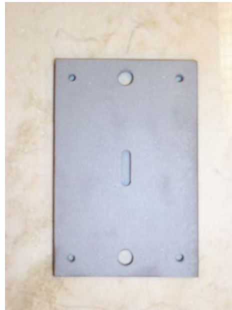
(b) Slotted defect
