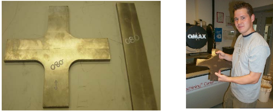
Figure 2: (a) Test specimens provided by Shell, (b) fabricated in-house.
