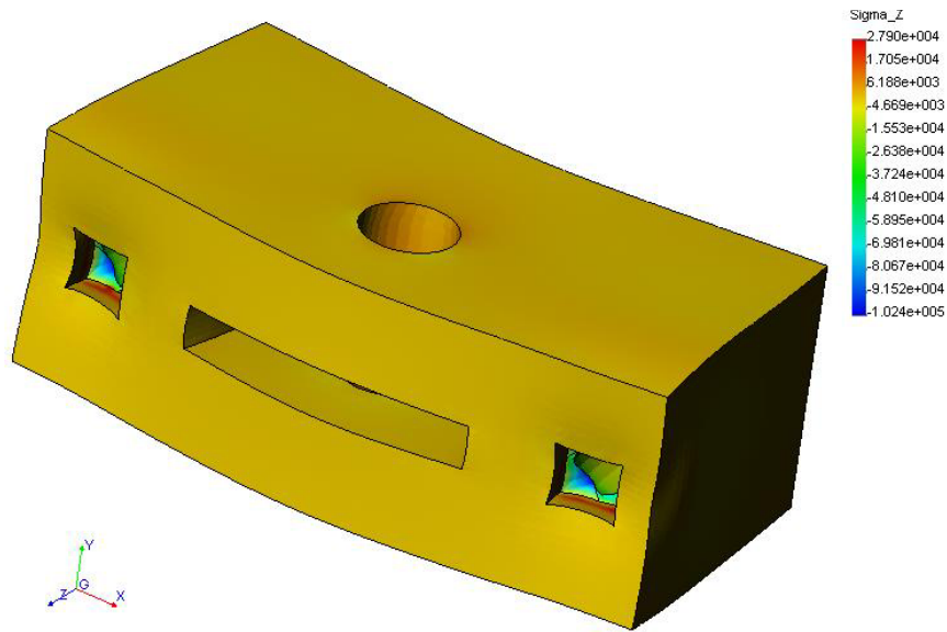
Figure 16: FEM analysis of the design of the loading clamping block.
