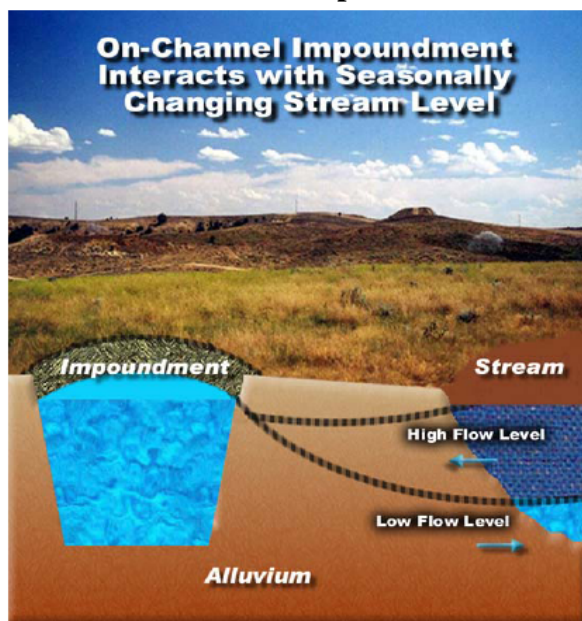
Figure 1-4: Schematic Diagram of On-Channel Impoundment
