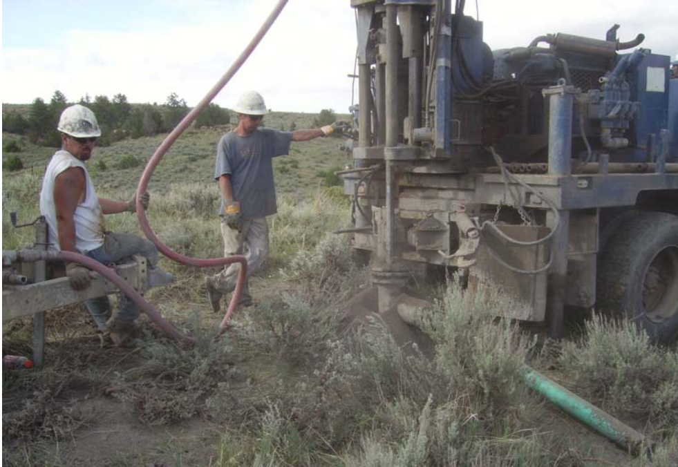
Air Rotary Drilling Boreholes and Monitoring Wells at CBNG Impoundments PRB, Wyoming
