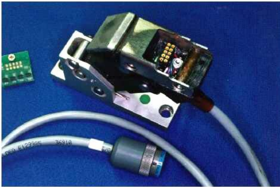
Figure 21. A sensor head with replaceable sensor circuit.
