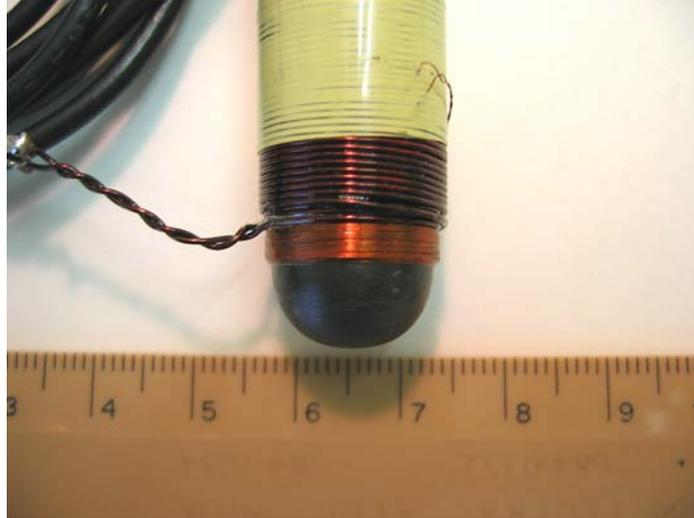
Figure 8. NLH probe with single rounded pole for reducing effects of probe tilt
