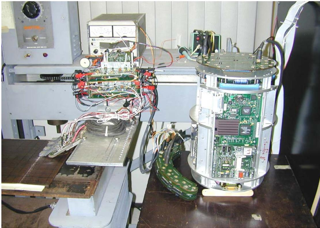
**Figure 24. NLH test setup with Linalog® MAX recorder and MUX unit**
