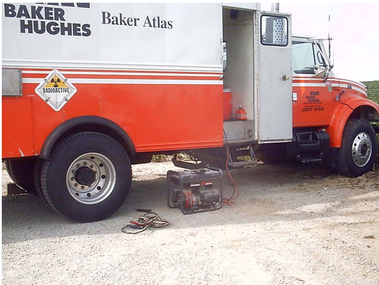
Figure 9: Wire line truck and separate external power generator
