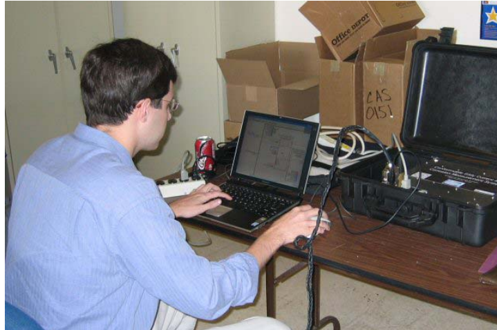
Figure 29. Laptop and suitcase may be conveniently located anywhere within 15 m of the pipe
