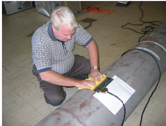
Figure 28. Contiguous areas are scanned in sequence under prompting from system software
