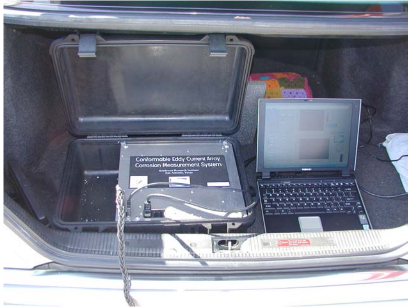
Figure 20. Control box and laptop computer deployed in the trunk
