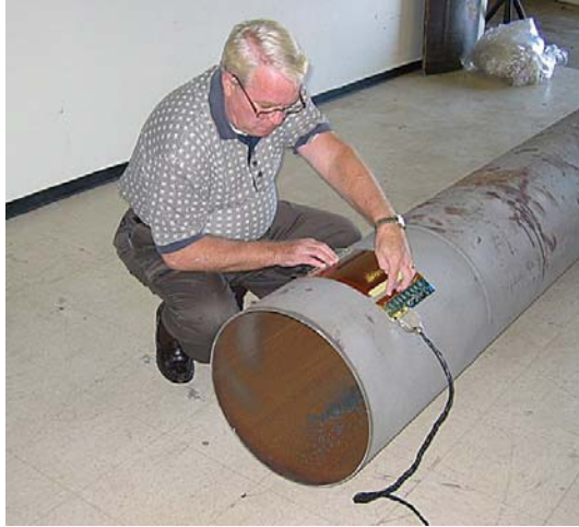
Figure 27. Baseline scans are taken on a smooth section of pipe surface
