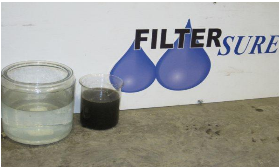
Figure 4: Effluent (left) following EC treatment and FilterSure filtration of Marcellus Shale FRW (right)
