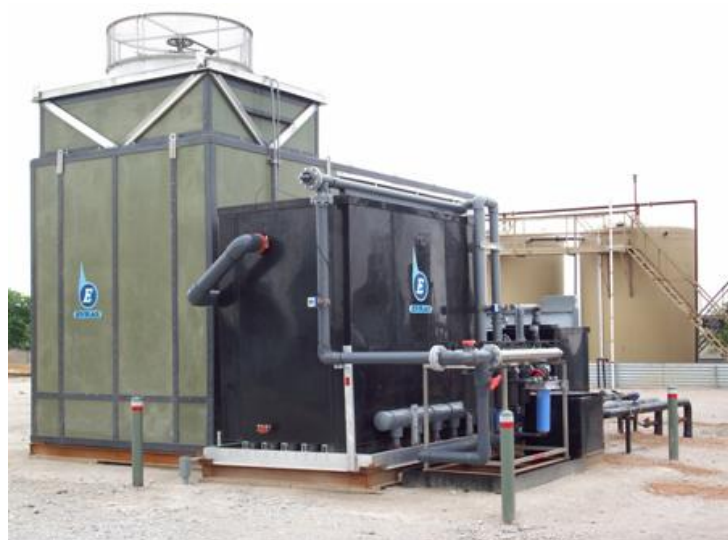
Exhibit 8. Evras Zero Discharge System for Produced Water
