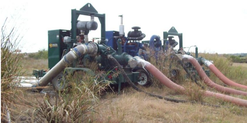
Exhibit 5. Industrial Pumps for Transporting Water via Temporary Pipelines
