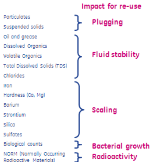
Figure 27. Key contaminants in frac flowback water and their impact on re-use in hydrofracturing.
