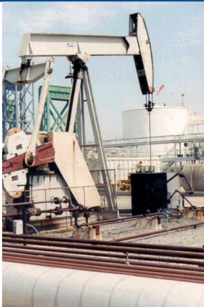
A pumpjack working in giant Wilmington oilfield in the Long Beach, CA, area. The large, wrapped pipeline in the foreground is a steamline.
