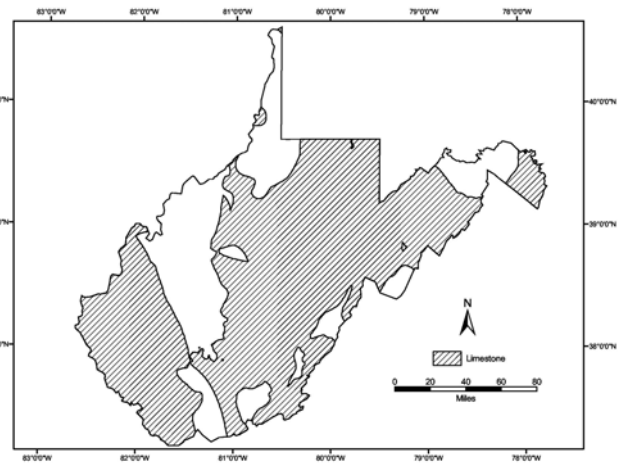
Figure 11. Limestone in West Virginia that is in the 6000 to 8000 ft depth range and over 300 ft in thickness (Units 3, 5 and 6).
