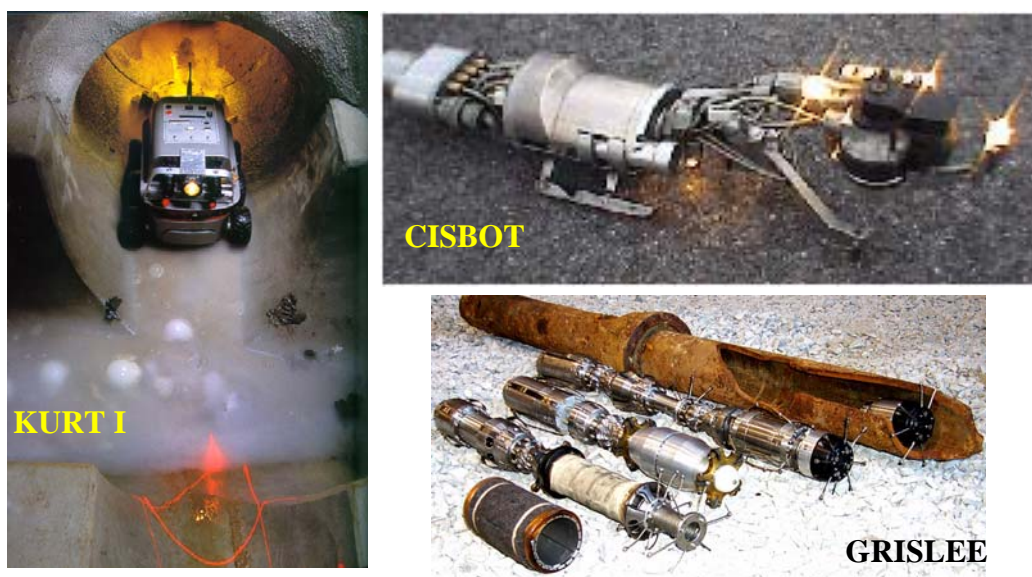
Figure 2: Tethered gasmain (CISBOT; GRISLEE) and untethered (Kurt I) robots
