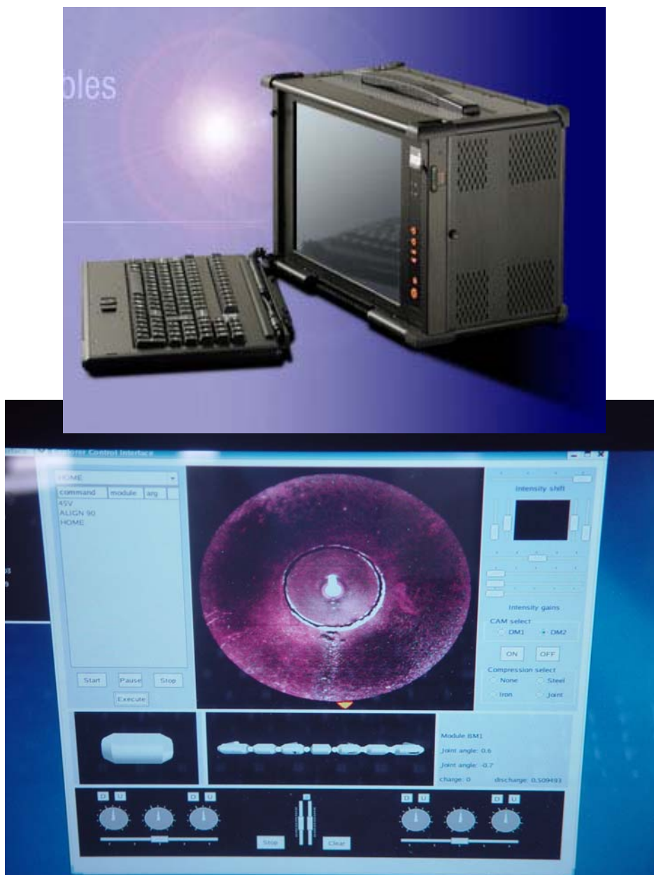
Figure 22 :Fisheye and dewarping imagery user interface with hardware platform
