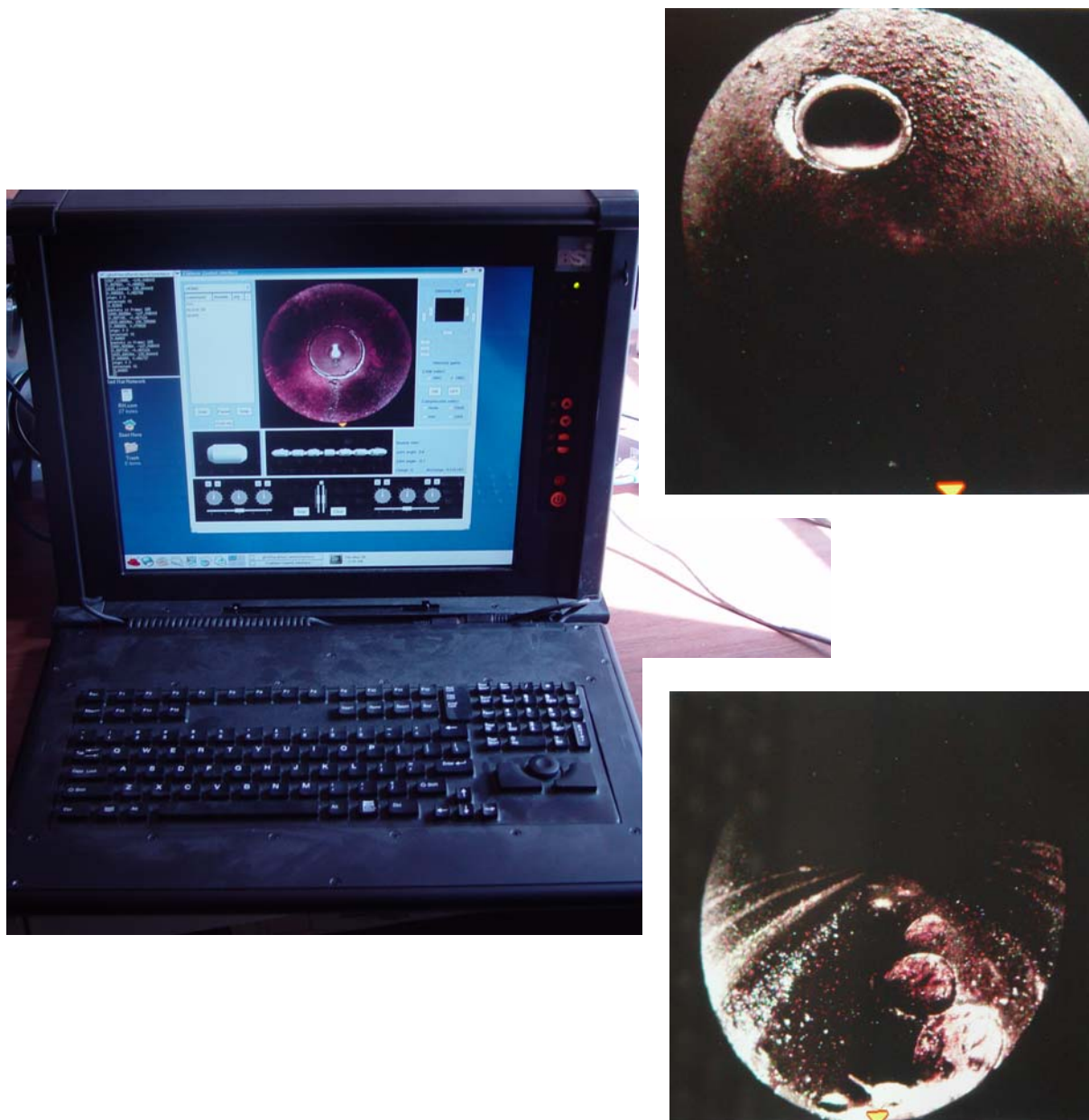
Figure 32 : Operator Interface & visible features (tap, bottle-caps, wheel-tracks)
