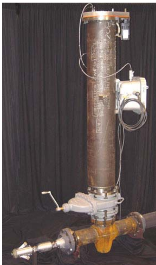
Figure 23 : Live-access launching hardware systems: Low-pressure CI and high-pressure steel
