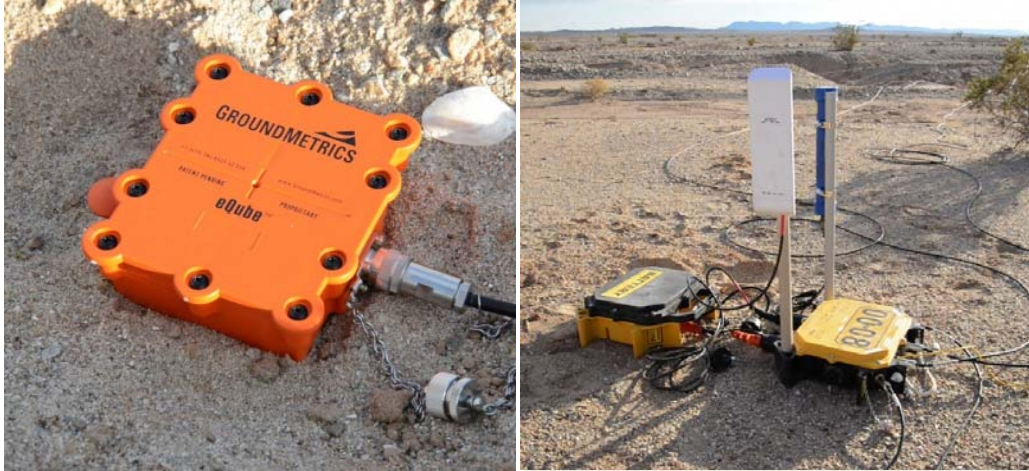
Figure 14. Sensing equipment. Left: Most recent sensor. Right: Data acquisition unit
