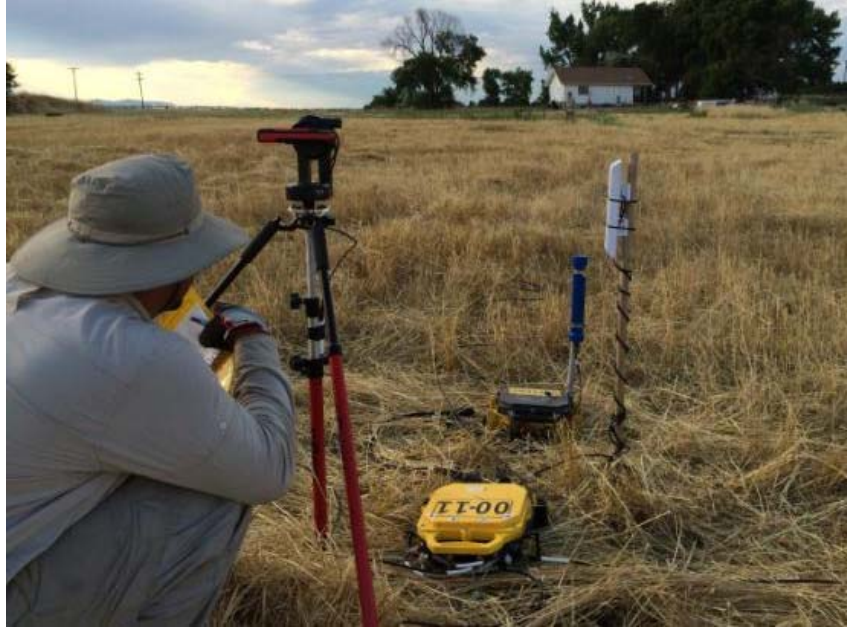
Figure 18. Using 4-way laser to line up orthogonal dipoles
