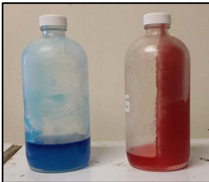
Figure 48: THF/water mixtures placed in laboratory refrigerator. The bottle on the left has solid crystals that have little or no blue dye in them. The bottle on the right has all crystals with red dye in them. The red dye will not be used in experimentation.
