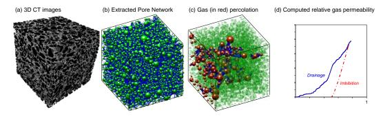
Figure 6: Pore network simulation based on 3D CT images. (a) Obtained 3D CT scanning images of the sands from the Mallik hydrate site. (b) Extracted stick-ball model of the pore network based on the CT images. (c) An illustration of the gas percolation path through the network. (d) Relative gas permeability during the drainage (gas invading water-saturated pore network) and the imbibition (water saturates a dried pore network) processes.
