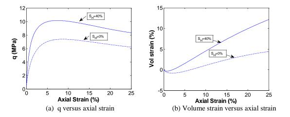
Figure 53: The stress-strain behavior of a soil under strain controlled test with hydrate saturation unchanged.
