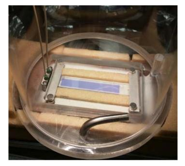
Figure 60: Humidity chamber with "house" supplied dry air continuously flowing.
