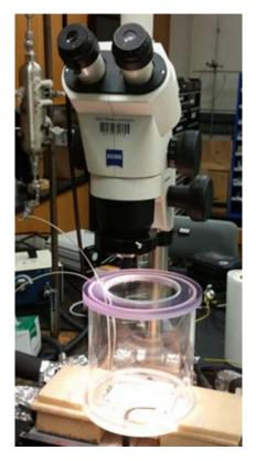
Figure 61: Humidity chamber installed over the chip and under the microscope.
