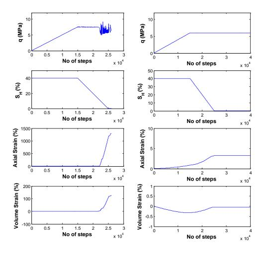
(a) Shear to q=7.5 MPa then dissociate (b) Shear to q=6 MPa then dissociate
