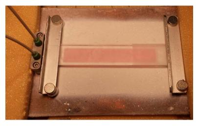
Figure 47: THF/water flow test in the microfluidic chip. Note the magnetic hold-down assembly and the white background on the copper bar.
