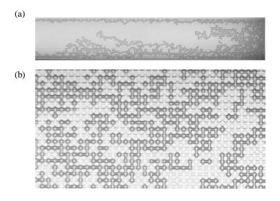
Figure 55: Microfluidic porous chip. (a) Water injection into dried microfluidic chip: image across the whole chip. (b) Ice nucleation in patches within the partially water saturated chip. White grids: ice saturated tubes; black grids: air saturated tubes.
