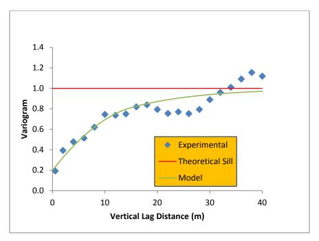
Figure 24: Experimental vertical variogram and model.
