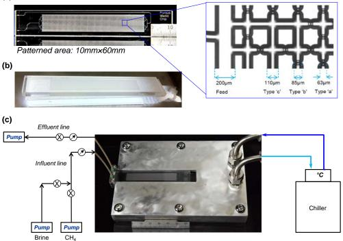
Figure 41: Microfluidic porous chip (a) porous space pattern, (b) illumination system, and (c) customized temperature control system.
