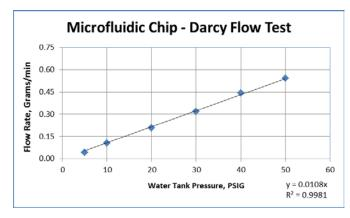
Figure 8: Darcy flow test results.
