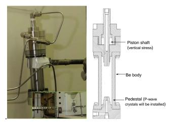
Figure 7: The Be vessel with two new endcaps are under leak test.
