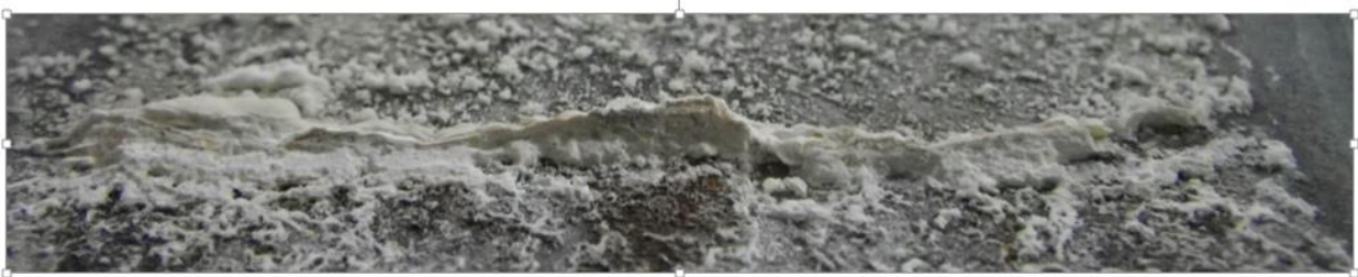
Figure 4. Calcium carbonate distribution within the 0.20 mm gap.
