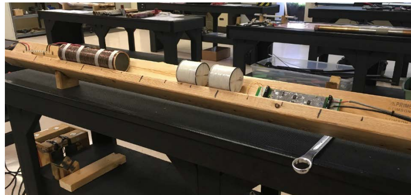
Initial bench testing of TX-RX coil setup
