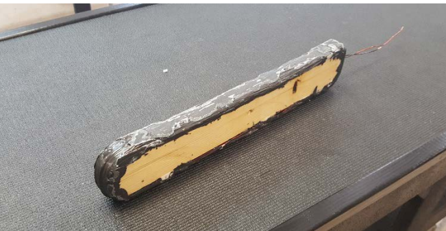
Co-planar coil after construction
