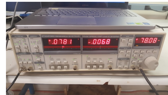
SR830 DSP Lock-in-Amplifier
