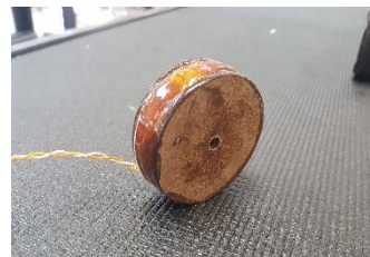
Initial bench testing of TX-RX coil setup
