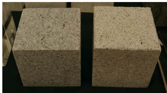
(c) Phase-transition-induced cracks in granite (block on the right was heated above the \alpha - \beta quartz transition point)
