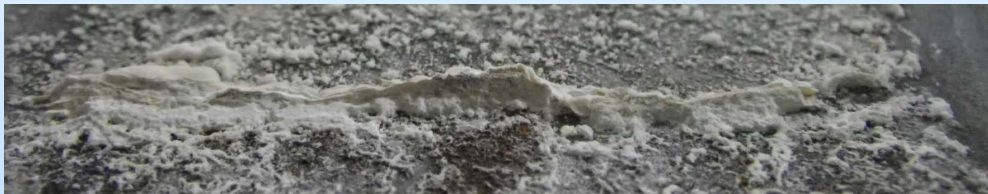
Carbonate seal on cement side of the fracture fixture formed right at the interface of the 0.2mm gap
