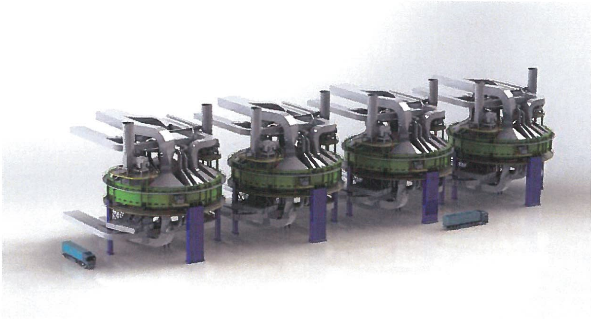
Exhibit 7-9: General Arrangement of VeloxoTherm™ RAMs for Case 12V (550MWe SC PC Installation)
