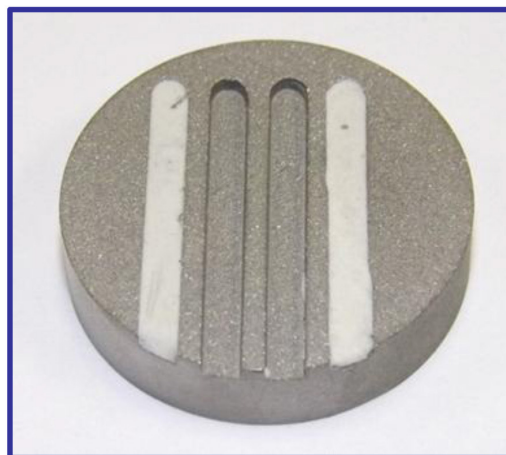
Figure 4. Ames Laboratory Grit Blasted Near Surface Embedded Micro-Channel Concept after Impregnation with Fugitive Thermoset Filler along the External Channels.
