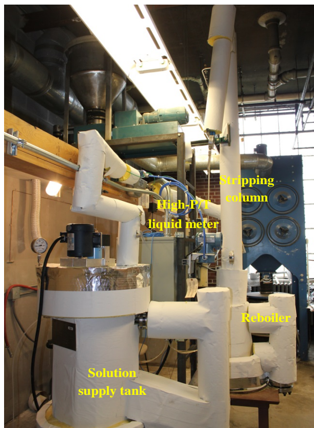
An existing stripping column rated at 200°C /500 psia
