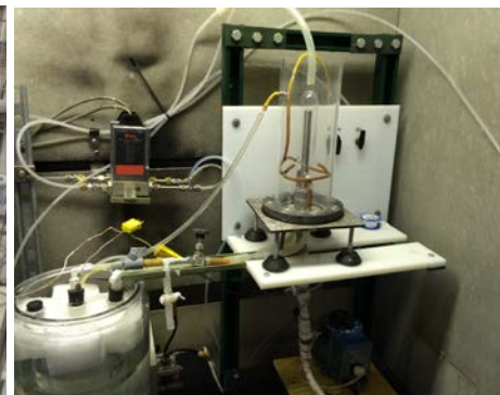
WWC reactor for kinetics
