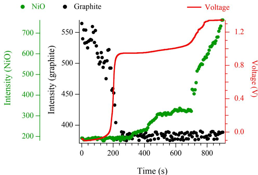
Operating at constant current leads to sequential changes in spectra that correlate with cell voltage
