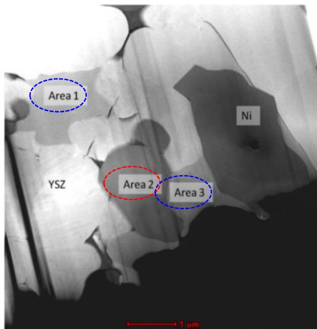
High resolution TEM/EDS image of Ni/YSZ sample impregnated with Al<sub>2</sub>TiO<sub>5</sub> and then heated to 1400°C.
