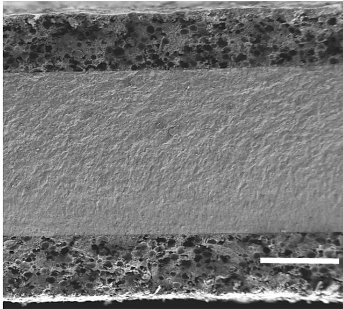
8YSZ electrolyte supported SOFC, bar = 100  $\mu\text{m}$
