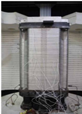
Current Pre-Commercial Integrated Manifold (PCI) Stack
