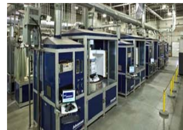
33 Test Stations: Single Cell to 25 kW Stack Testing
