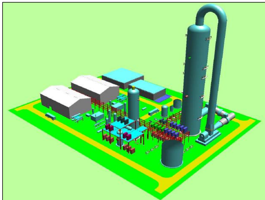
3D model for SIH 1 configuration: blower downstream of absorber column and combined DCC and absorber
