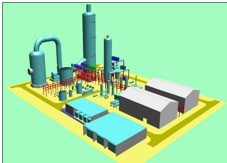
3D model for SIH 2 configuration: blower upstream of absorber column and separate DCC and absorber
