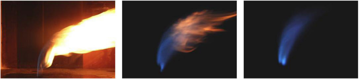
Figure 1. Jet flames in crossflow with different levels of premixing. The fuel is 70% \text{CH}_4 + 30% \text{H}_2 . From left to right: non-premixed, jet fluid diluted by 25% (volume basis) with air, and jet fluid diluted by 50% with air.
