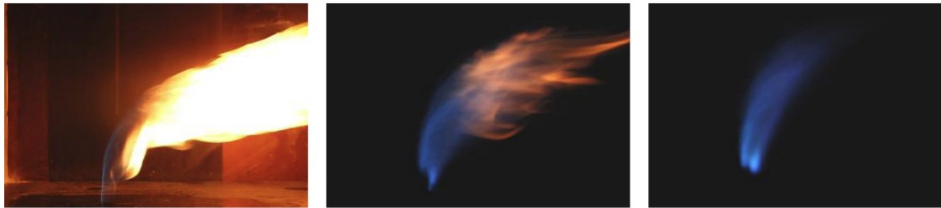
Figure 12: Jet flames in crossflow with different levels of premixing. The fuel is 70% CH 4 + 30% H 2 . (a) non-premixed, (b) jet fluid diluted by 25% (volume basis) with air, and (c) jet fluid diluted by 50% with air.
