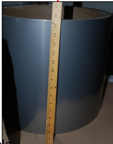
15" wide, 4 mil AFA foil for Solar Turbines (foil by Elgilo)y
