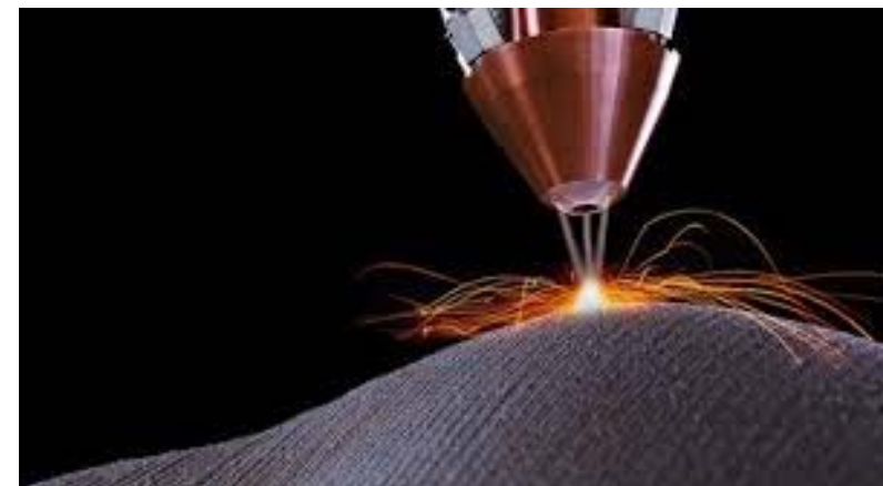
LENS: Laser Engineered Net Shaping
