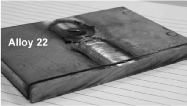
Alloy 22 FSW showed only very fine intergranular TCP phases – no large grain boundary phases
