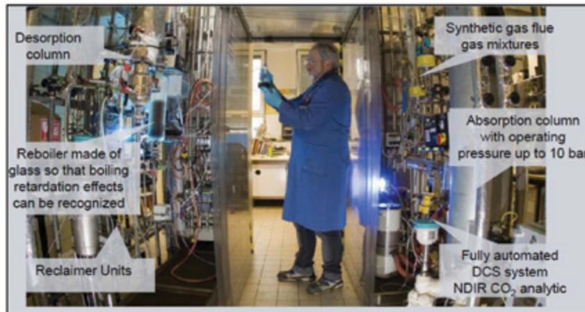
Figure 1: Siemens Lab Plant for CO<sub>2</sub> Capture Tests at Frankfurt Hoechst Industrial Park
