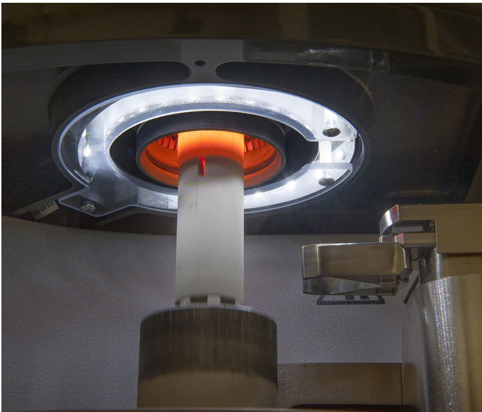
Oxygen/Nitrogen by Inert Gas Fusion Infrared and Thermal Conductivity Detection
