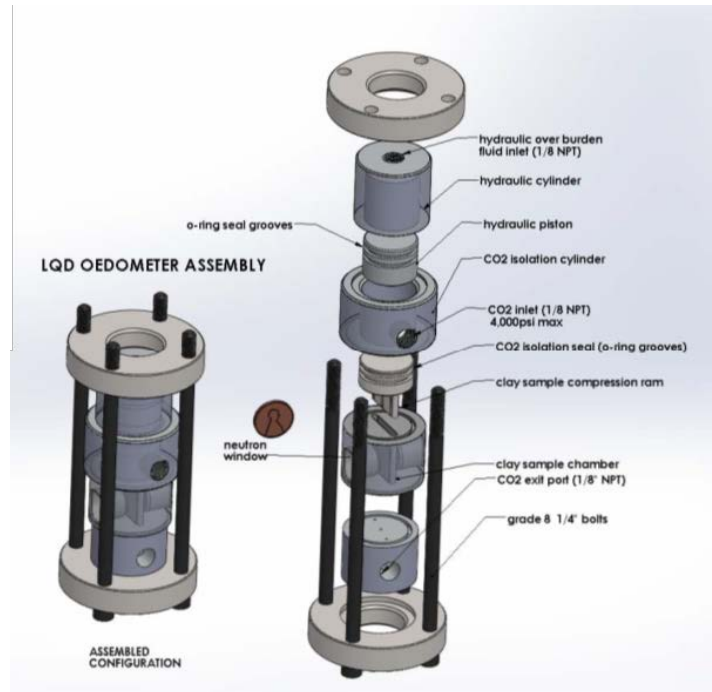
Figure 11: Stainless steel/aluminum oedometer using small angle neutron beam scattering to observe caprock swell with supercritical CO 2 .
