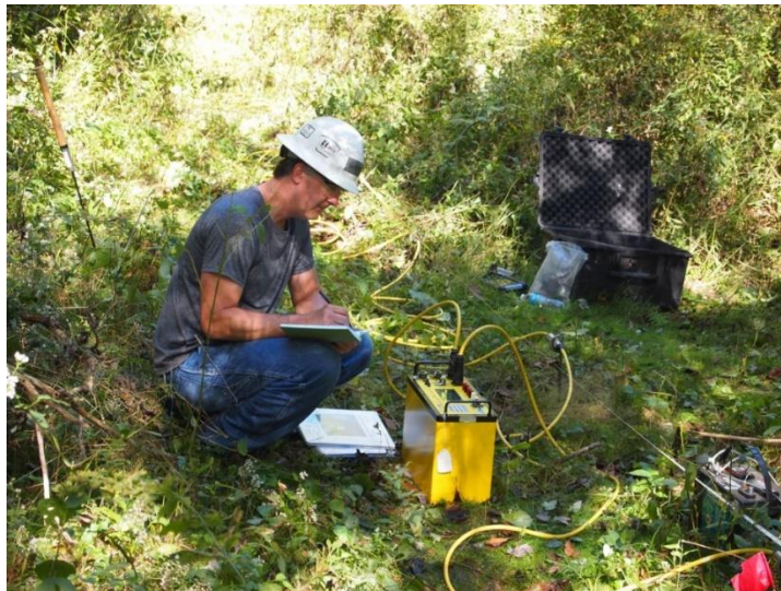
Figure A4: NETL Researcher operating a resistivity instrument over a suspected abandoned well appearing in the PA/IRIS/WIS database. The record for this 1902 well describes it as a dry hole having a section of casing lost at an unknown depth during a salvage-for-reuse operation. These data were inversion-modeled to estimate the depth to the top of the well casing.
