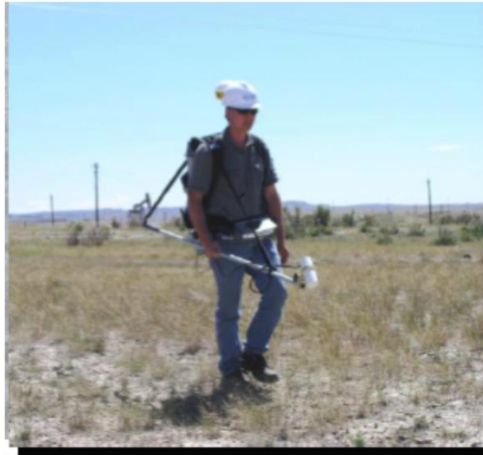
Figure 1: Ground-based survey employing a GPS-linked cesium-ion magnetometer.
