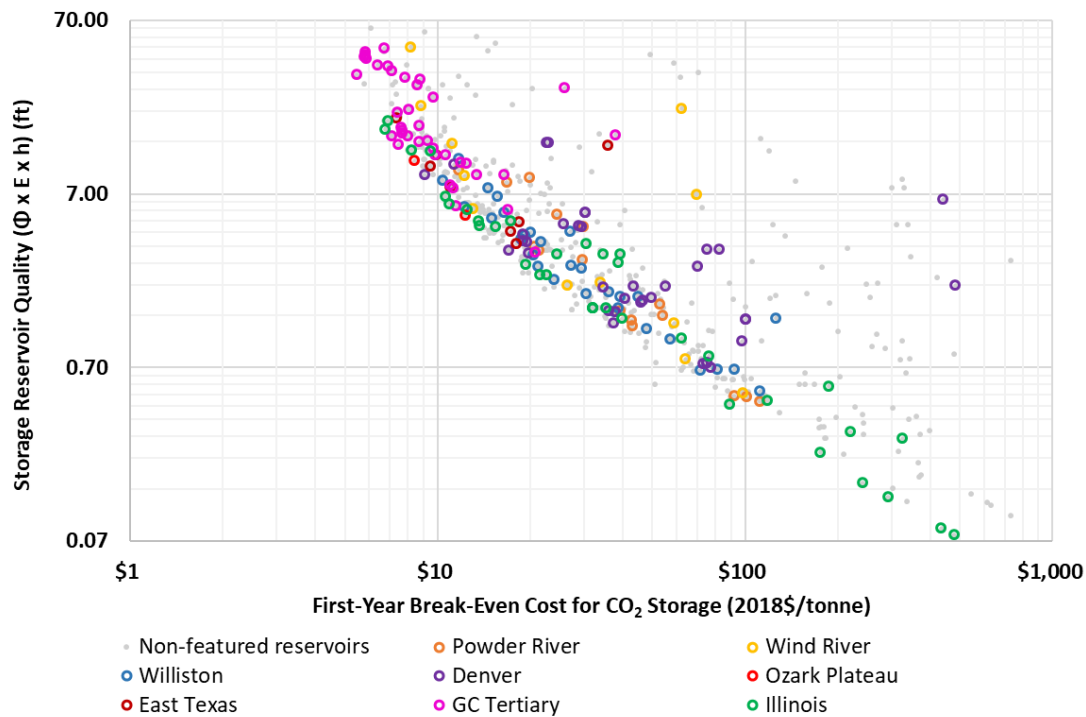
Exhibit 3-3. Storage reservoir quality against CO 2 break-even storage cost for SCPC plant (4.33 Mt/yr capture rate) highlighting basins of selected storage reservoirs in dome and regional dip structural settings
