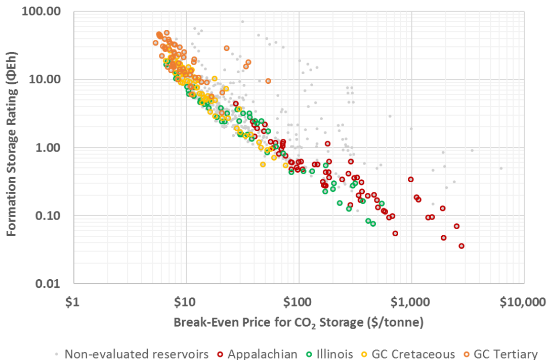
Exhibit 3-12 Basin characteristic against CO 2 break-even storage price for electric power plant (3.58 Mt/Yr capture rate)
