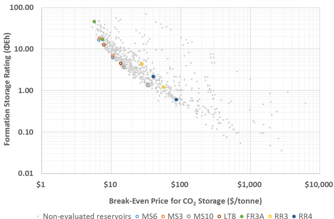
Exhibit 3-13 Reservoir characteristic against CO 2 break-even storage price for electric power plant (3.58 Mt/Yr capture rate)
