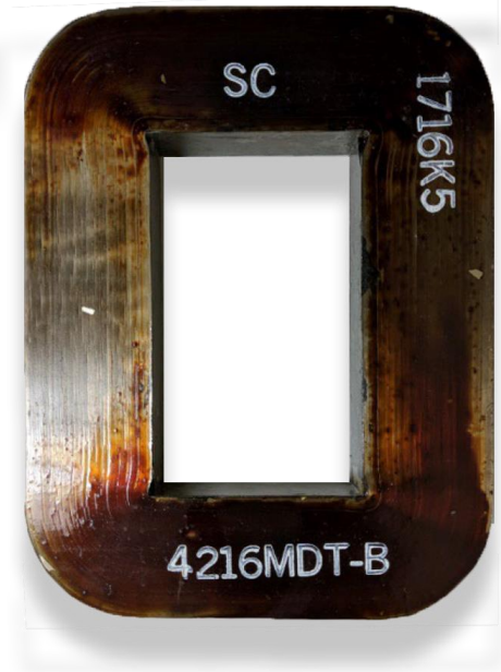
Fig. 1: Core under test (Nano-crystalline core).
