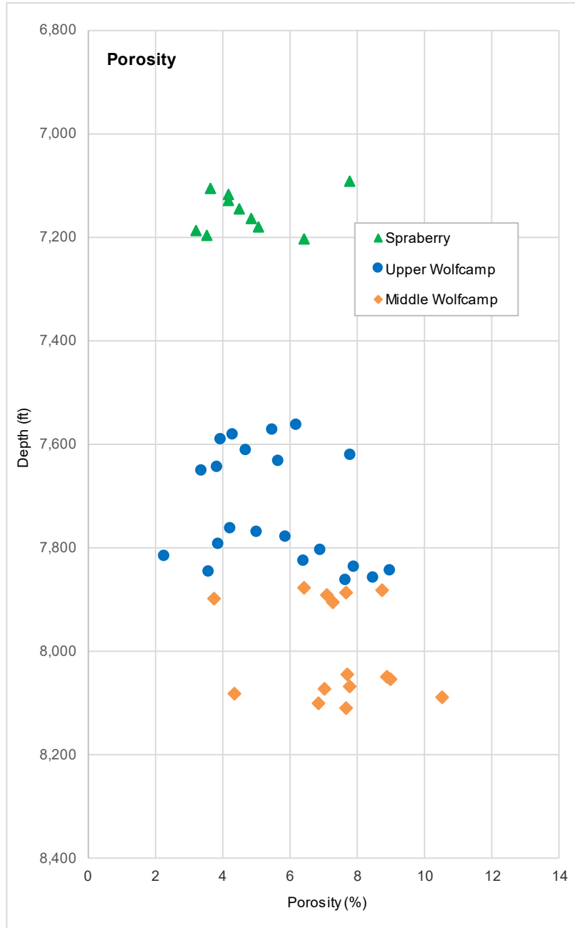
Figure 20: Porosity from MR testing in vertical pilot well SUGG-A #171 7SU.
