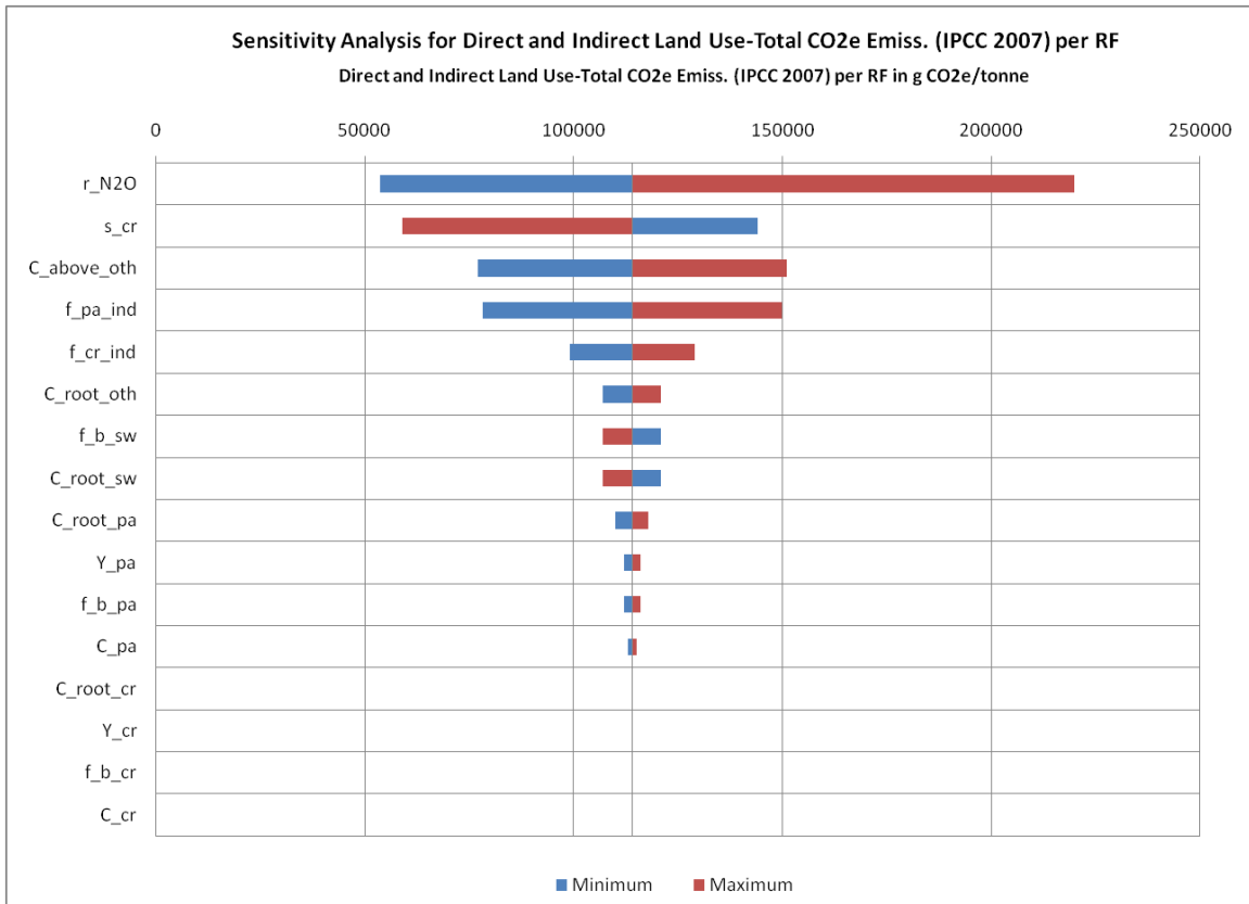
Figure 23. LC Stage #1c Sensitivity Analysis Results for Total CO 2 e Emissions for Direct and Indirect Land Use Changes (Using IPCC 2007 GWP) (g CO 2 e per Tonne Switchgrass Ready for Transport)
