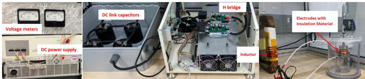
Figure 3: Insulation characterization system lab setup.
