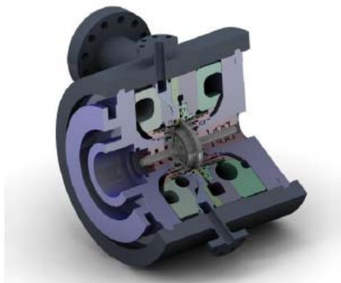
Exhibit 4-8 Ramgen Single-Stage, Direct-Drive HP Configuration
