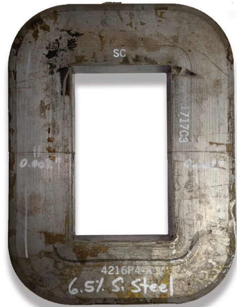
Fig. 1: Core under test (6.5% silicon core)
