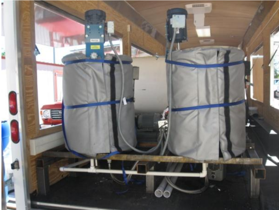
Figure 21: Placement of the mixing tanks in the trailer
