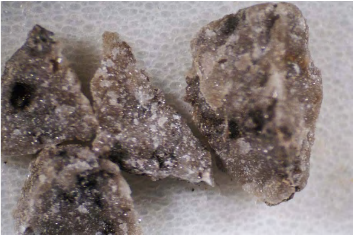
Binocular microscope image (1400x) – Pure Big Flat 3 (Map #19), 7716-17 feet, four representative samples used for grading showing tight white dolomite.
