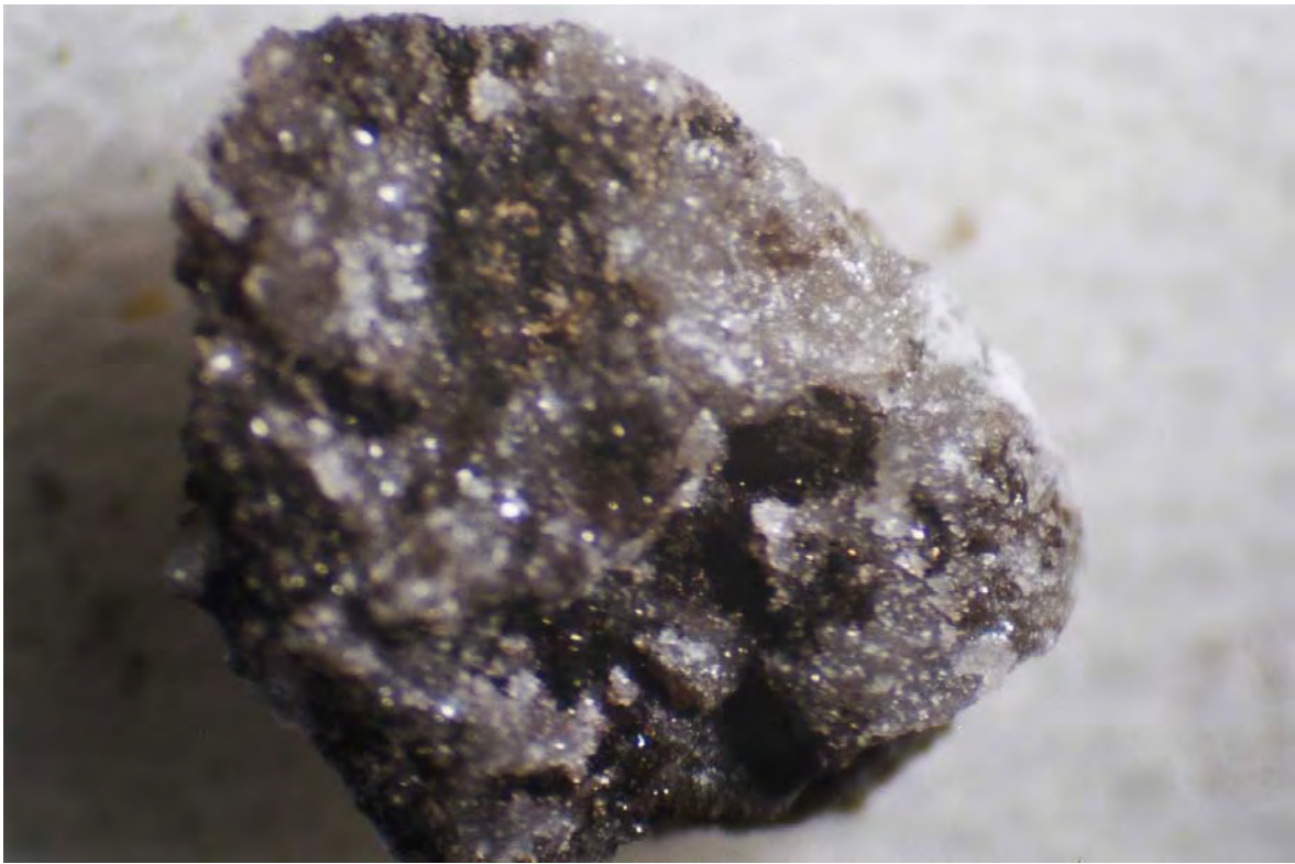
Binocular microscope image (3000x) – Pure Big Flat 3 (Map #19), 7715-16 feet, representative core chip with moldic/microvuggy porosity and bitumen (plus drilling mud).
