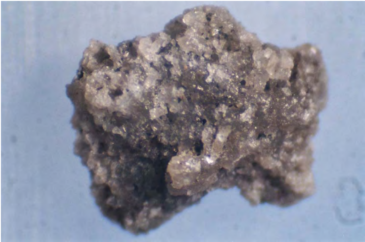
Binocular microscope image (4500x) – Pure Lisbon 814-A (Map #31), 8900-05 feet, single dolomite cutting with intercrystalline porosity and traces of bitumen.
