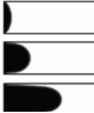
Figure 18. Simulations of fluid displacement for increasing difference in pressure controlled by the density at the outlet. Values from top to bottom are: 0.2508, 0.2498, 0.2482 and 0.2466. D2Q9 lattice of size 35x130 lu 2 . Parameters for simulations are \bar{k}=0.1 , D_\rho=0.99 and \rho_l/\rho_g=10 ( \bar{k} defines surface tension).
