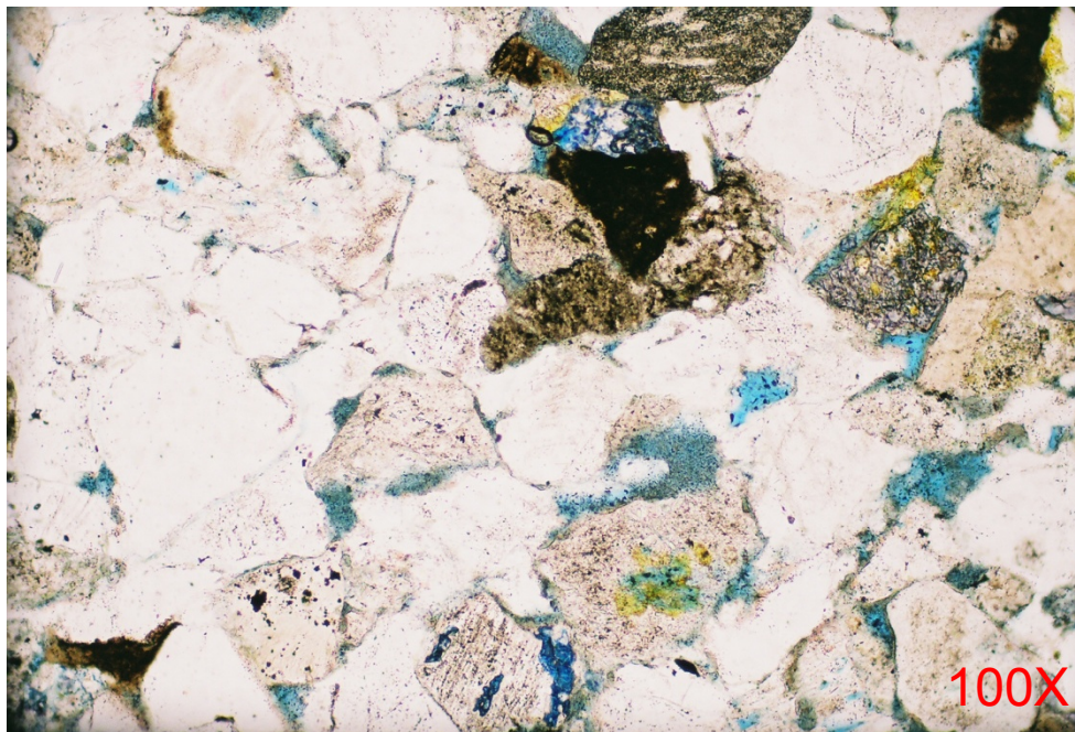
Figure 4.5.13. Example Mesaverde thin section for Type IV porosity. Porosity consists almost entirely of sparse, poorly connected, clay-filled intergranular microporosity. Quartz cement is prominent, ferroan calcite is sparse. Pore-filling clay cement causes elevated S_{wi} , reduced relative permeability and increased P_c entry pressure. Williams PA 424, 4686.4', Rock Type 15286, \phi = 7.9\% , GD = 2.65 \text{ g/cc} , K_a = 0.211 \text{ mD} , K_{ins} = 0.0031 \text{ mD} .
