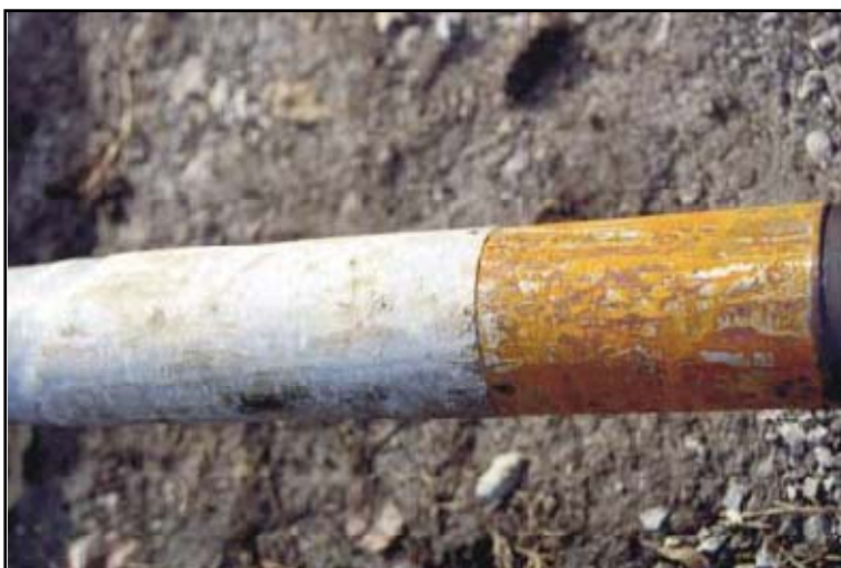
Figure 10. Condition of joint end after use—a little rust on the steel end, but the composite has only a few scratches.
