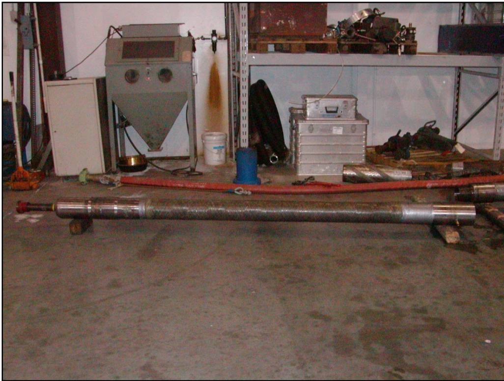
Figure 17. Composite pipe segment
