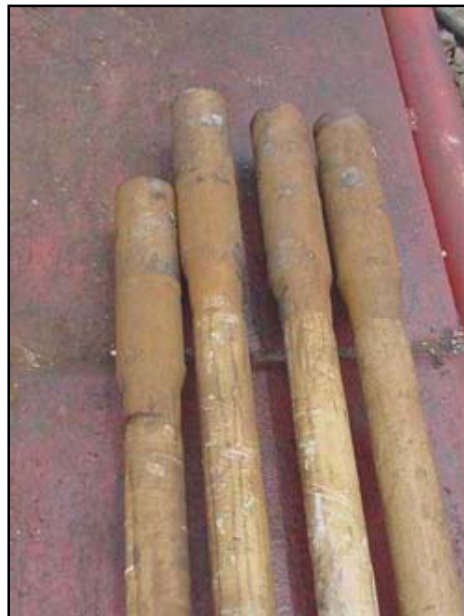
Figure 12. After 160,000 air hammer cycles, the composite drill pipe exhibits little to no signs of wear.
