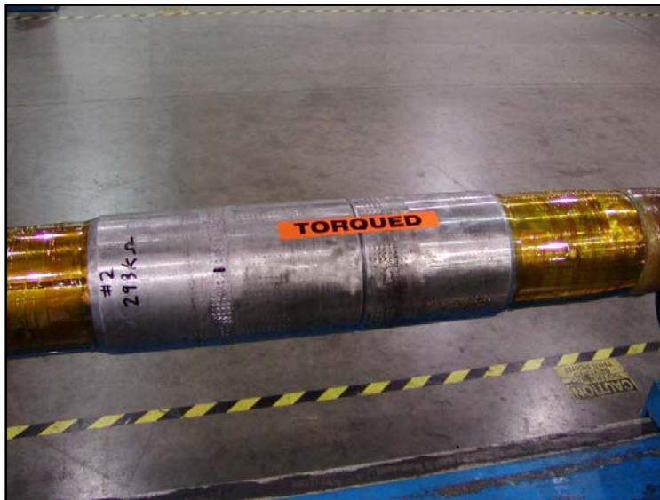
Figure 26. CDP made up to correct torque
