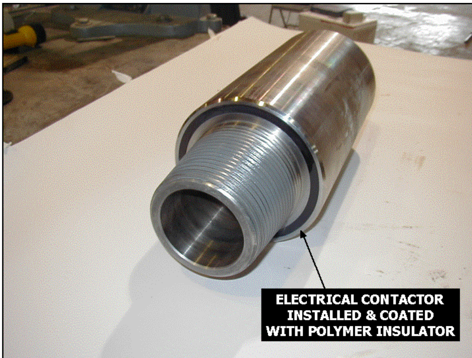
Figure 14. The 4-1/2 inch IF Pin connection fully assembled.
