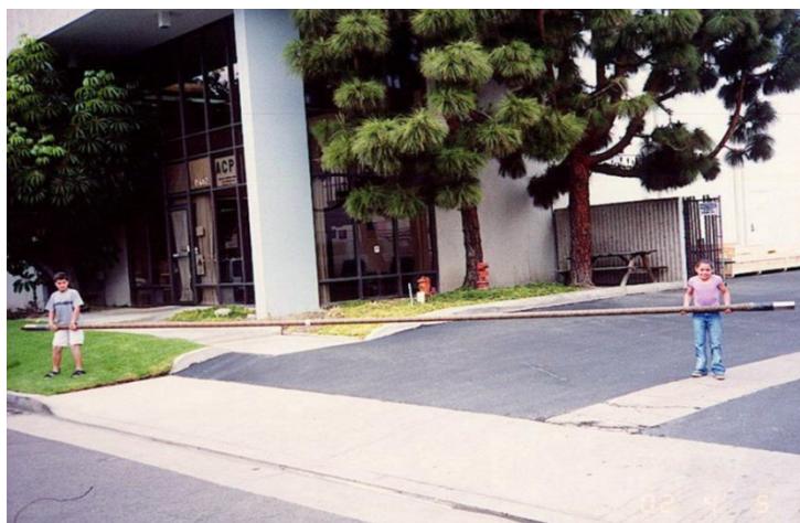
Figure 1. A 30 foot section of composite drill pipe is being carried by a 9/10 year old sister/brother team to demonstrate the light weight of CDP.
