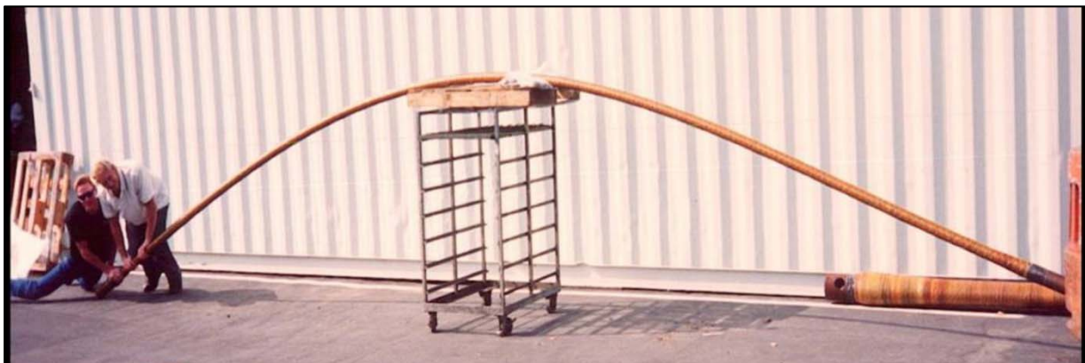
Figure 9. Short radius CDP is flexible enough to resist bending fatigue, but strong enough to carry 25,000 pounds of tension and 2,000 lb-ft of torque.
