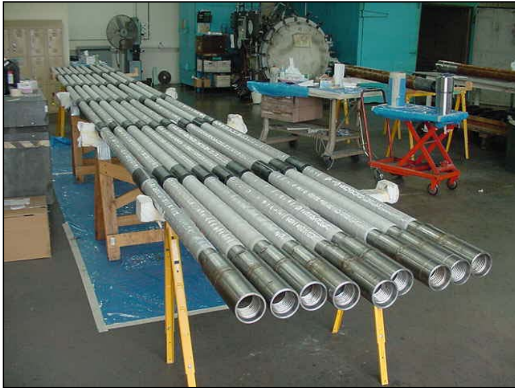
Figure 11. Short radius composite drill pipe delivered to J.B Drilling
