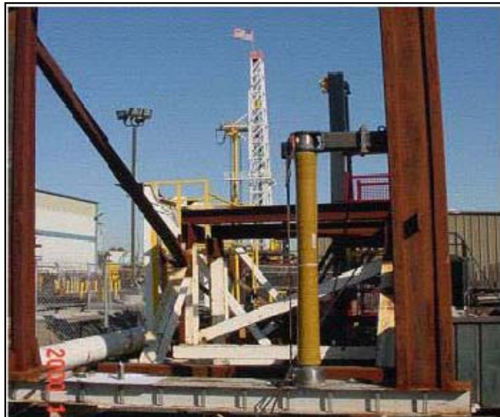
Figure 4. Ten-foot full diameter torsion test apparatus
