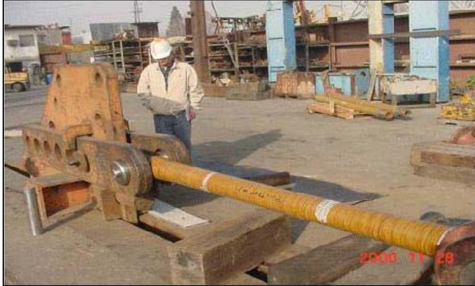
Figure 5. Ten-foot full diameter tension test apparatus
