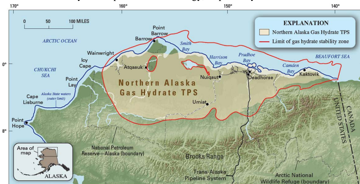
Figure 2: Northern Alaska Gas Hydrate Total Petroleum System (TPS) (shaded in tan), and the limit of gas hydrate stability zone in northern Alaska (red outline); USGS Fact Sheet 2008-3073.
