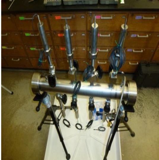
Figure 1 Instrumented Pressure Testing Chamber (IPTC) showing probe ball valves, drive arms, and the ends of the instrumented probes
