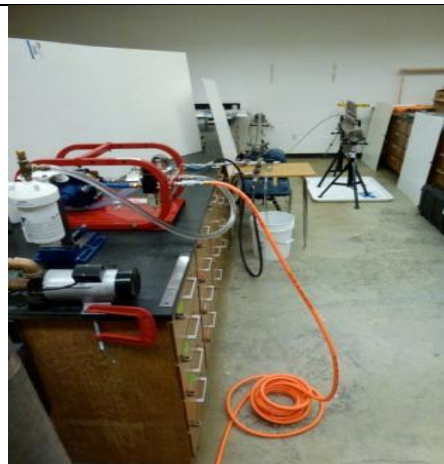
Figure 14 Pressuring the IPTC in Atlanta using a new pump and manifold system
