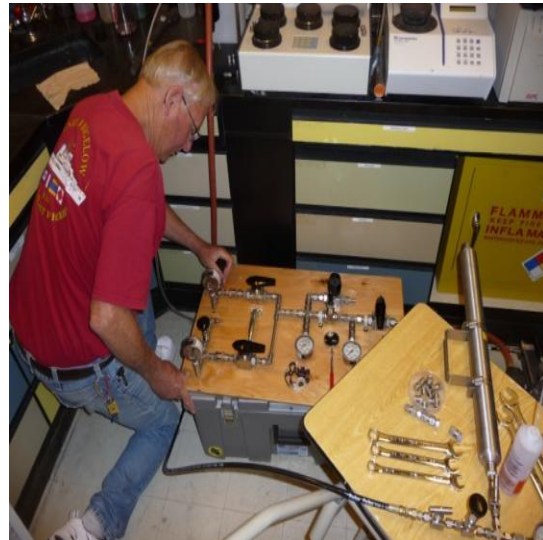
Figure 4 Dave Mason pressure testing a new manifold system
