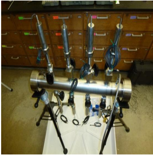
Figure 5 Instrumented Pressure Testing Chamber (IPTC) showing probe ball valves, drive arms, and the ends of the instrumented probes
