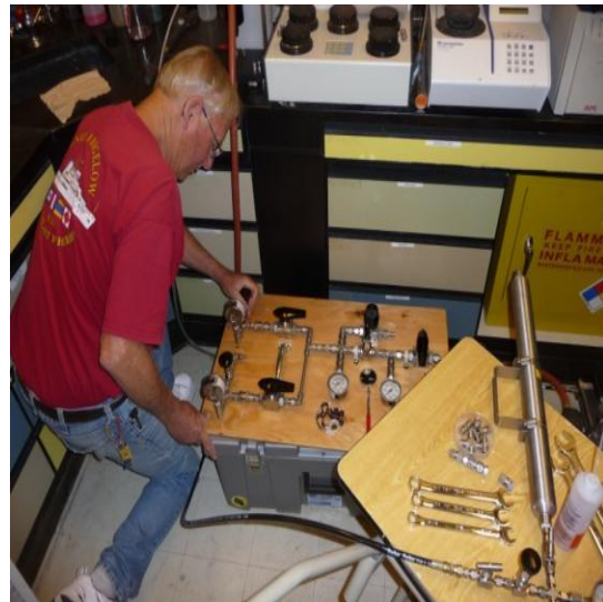
Figure 8 Dave Mason pressure testing a new manifold system
