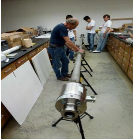
Figure 9 Manipulator string used to precisely move a core section through the IPTC
