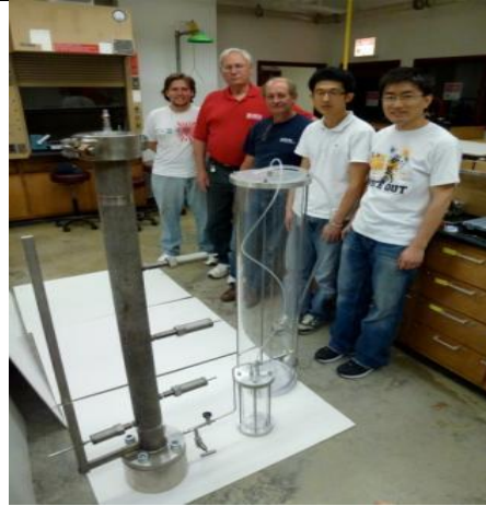
Figure 12 Depressurization System holds core. Water and gas collect in small and large clear containers.
